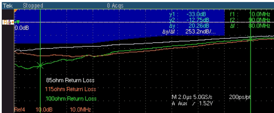
Figure 9-18: Waveform for 100BASE-TX Return Loss Transmitter
