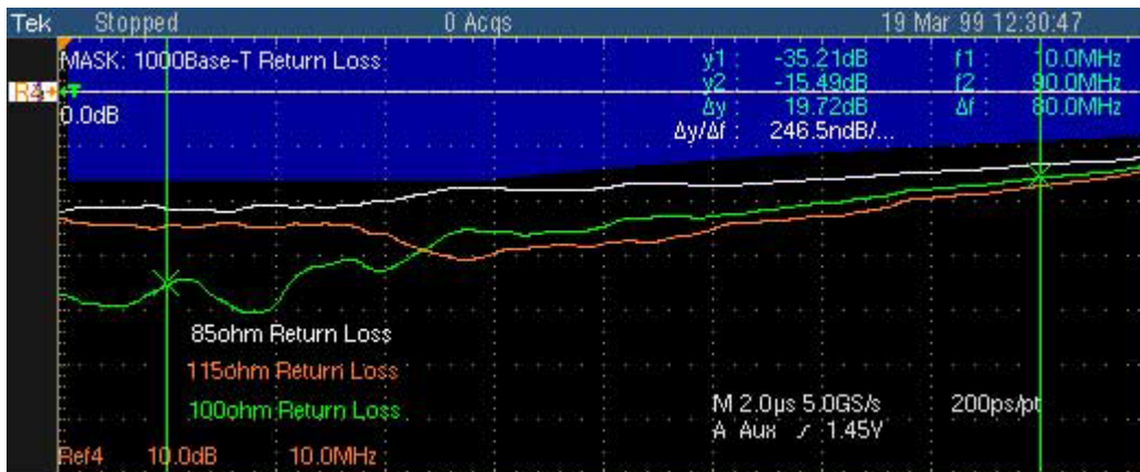
Figure 8-23: Waveform for 1000BASE-T Return Loss
