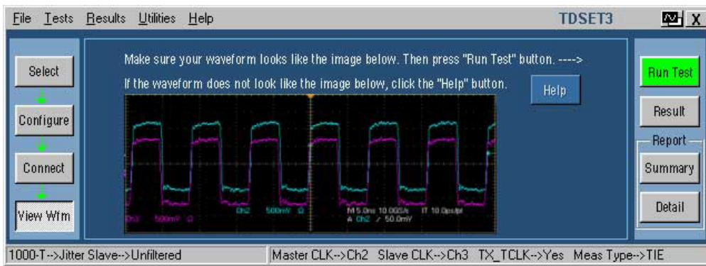
Figure 11-9: 1000BASE-T View Waveform for Jitter Slave Unfiltered (with TX_TCLK access)
