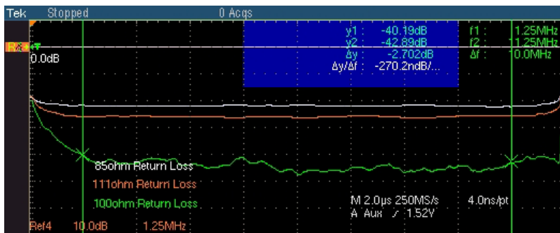
Figure 10-24: Waveform for 10BASE-T Return Loss Receiver
