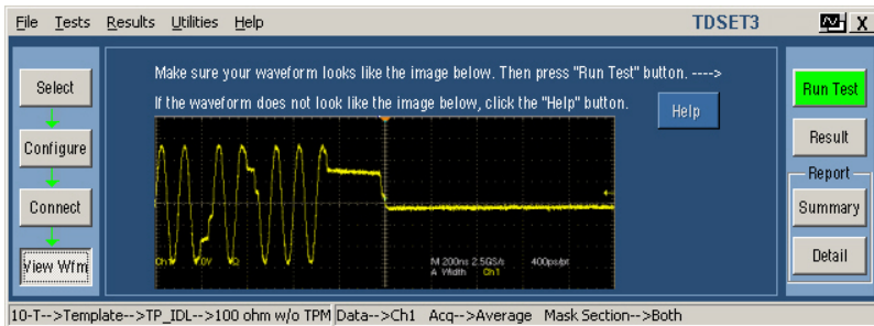
Figure 13- 3: 10BASE-T View Waveform for TP_IDL
