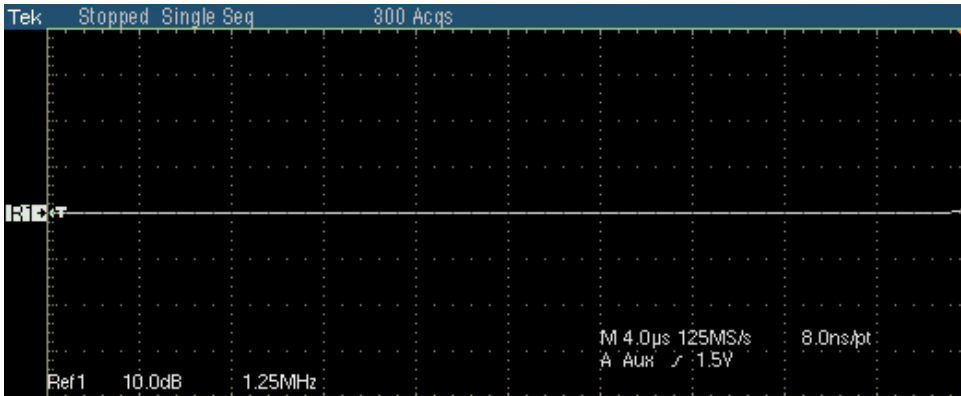
Figure 18- 19: Waveform of 10BASE-T Return Loss Open Calibration
