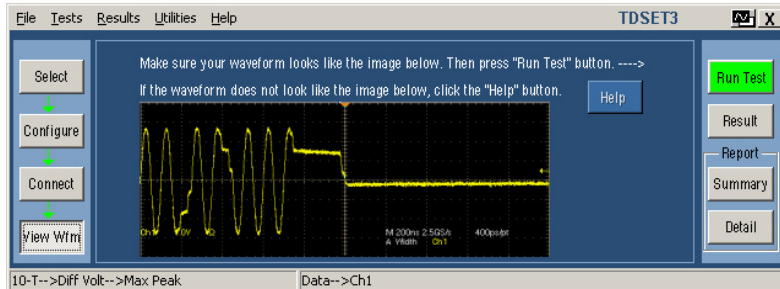
Figure 13-6: 10BASE-T View Waveform for Differential Voltage
