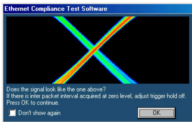
Figure 10- 15: 10BASE-T Jitter with cable user control
