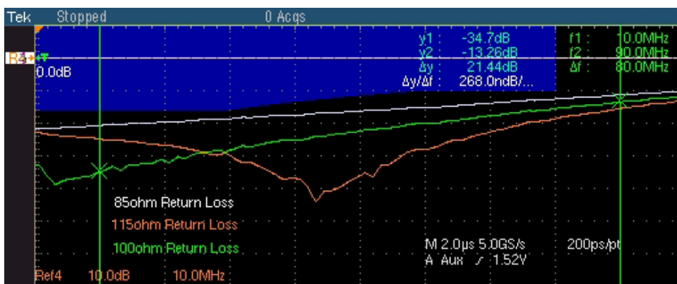
Figure 9-19: Waveform for 100BASE-TX Return Loss Receiver
